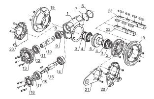
Fig 9.5.1/2 Spare parts-Worm gearboxes MRP
