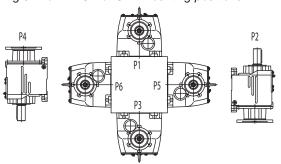
Fig 9.1.2/2 ATC Mounting positions
